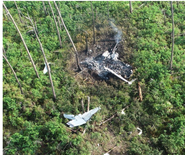
Photo 1: N790JR ground scars and post-crash fire at accident site
