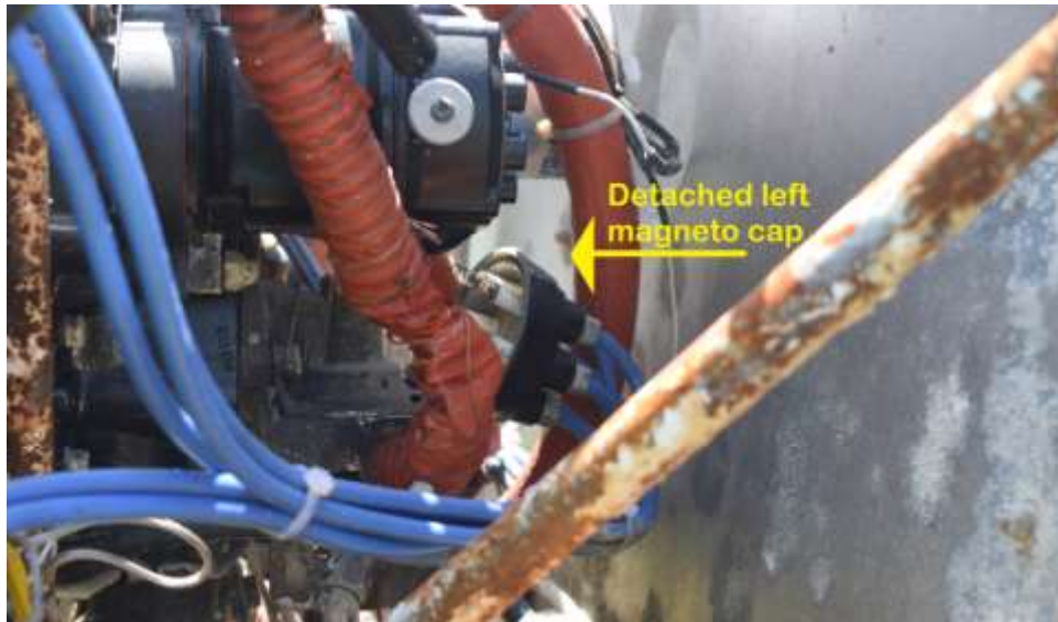
Fig. 5: Left magneto cap detached from housing
