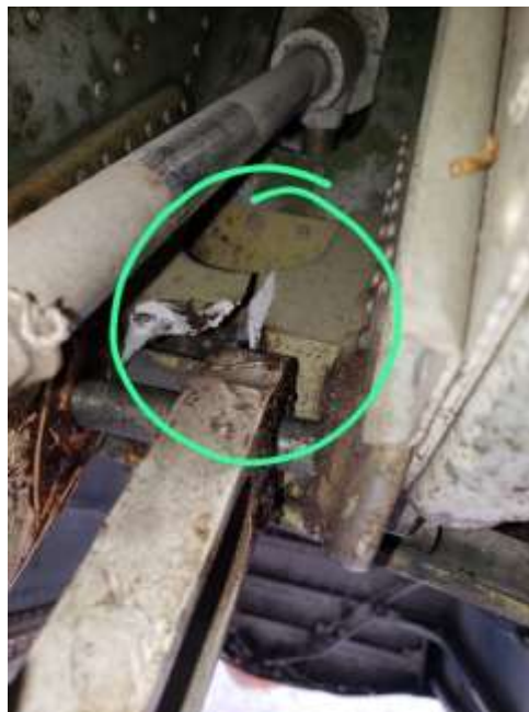
Fig. 3 Left main landing gear drag brace support fitting
