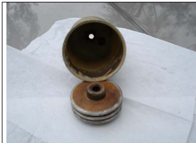
Left fuel strainer bowl found rusted, corroded and stained with sediments.
