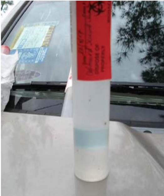
Water and fuel sample taken from right engine gaskolator. Taken on August 23, 2007. C6-LEE
