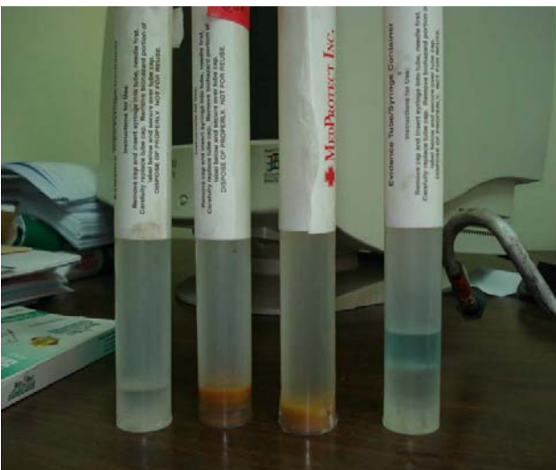
Fuel samples showing water dirt and other sediment retrieved from inspection of fuel lines, Gascolator and strainer of C6-LEE Left and right engine, fuel lines, Gascolator and spider valve.
