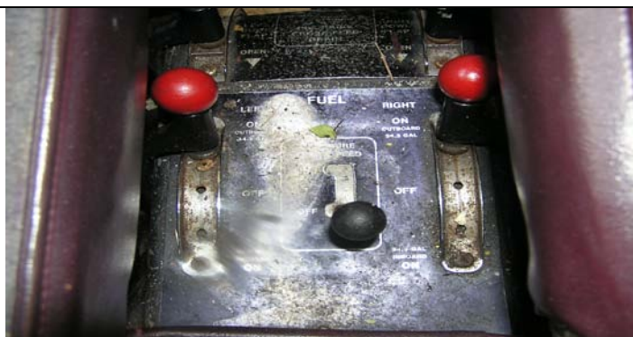
Fuel Manifold and Fuel Supply lines that were found contaminated with water and sediments. (Photo shows left engine only, however, both engines, and its associated fuel supply lines and flow dividers were found contaminated with water)
