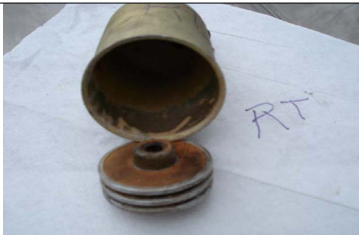
Right fuel strainer bowl found in the same sediment stained and corroded condition.
