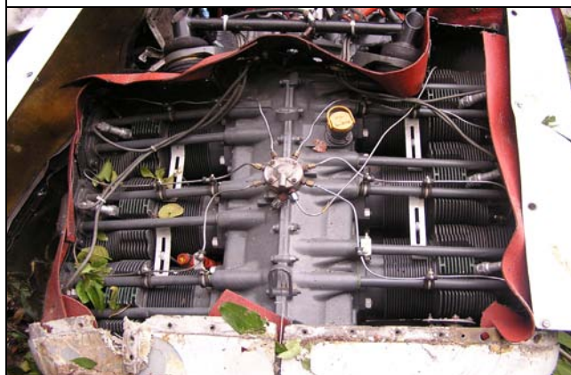
Fuel Manifold and Fuel Supply lines that were found contaminated with water and sediments. (Photo shows left engine only, however, both engines, and its associated fuel supply lines and flow dividers were found contaminated with water)
