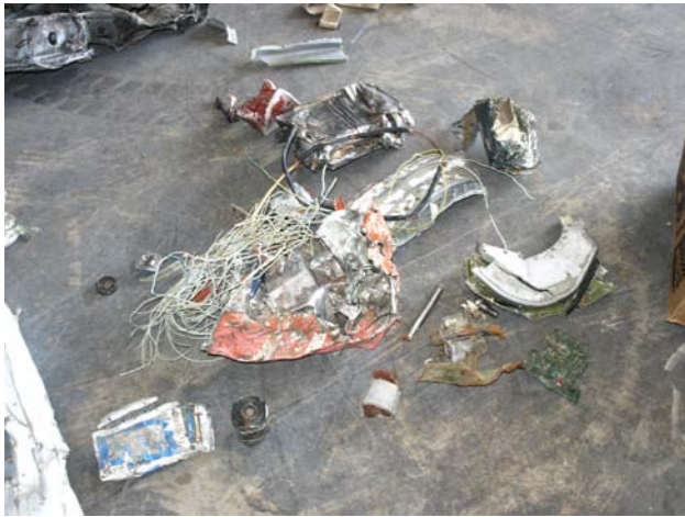
Figure 9 and 10. Actual CVR case recovered from N28RK. Case was destroyed internal parts and recorder never recovered.
