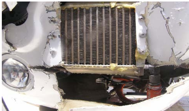
Damage sustained by the lower engine cowling
