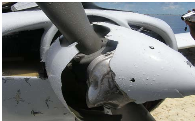
Damage sustained by the propeller dome.
