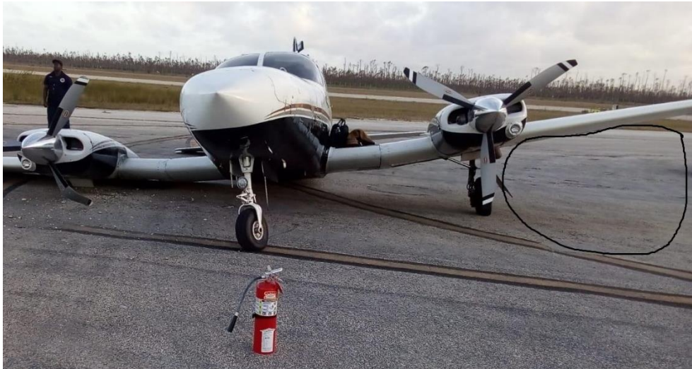
Area in circle and under left wing shows series of pothole on taxiway
